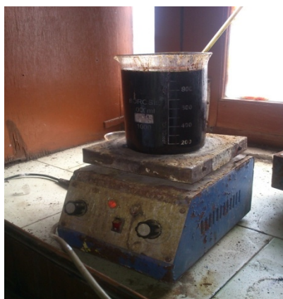
Figure-4.2 Heating of Neem oil by Magnetic Stirrer Heater
