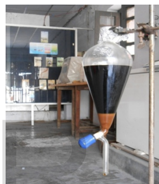
Figure-4.4 separation of NOME and glycerol
